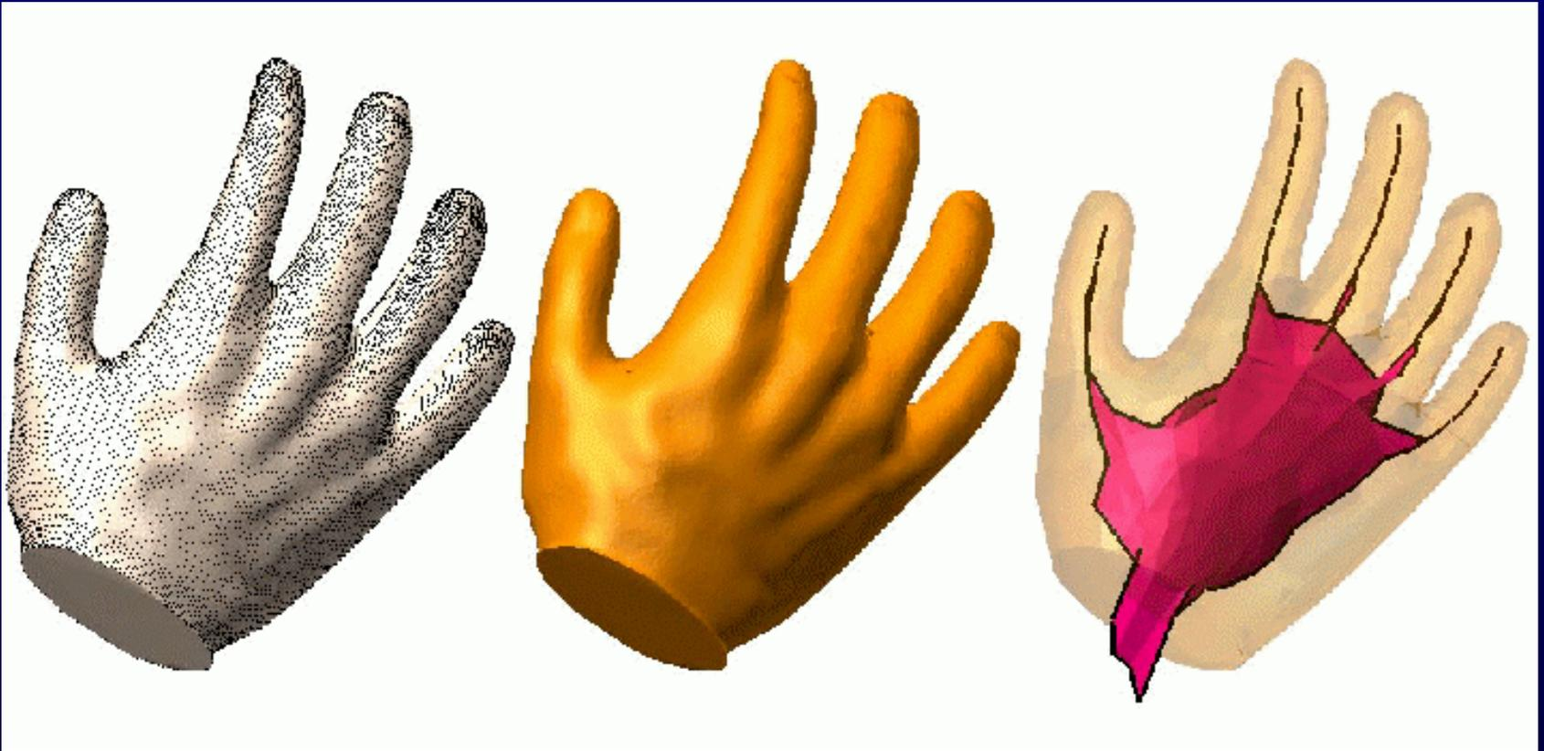
Laser range data, power crust, simplified approximate medial axis.
