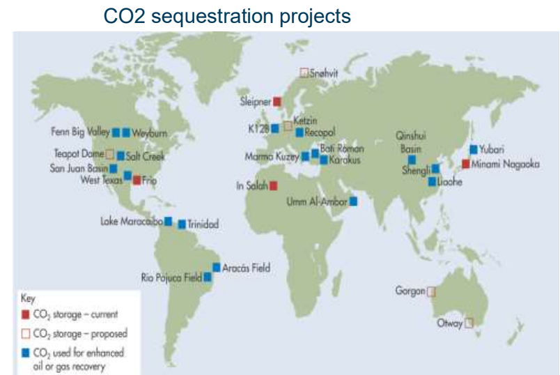
Location of sites where geological storage of CO 2 and CO 2 enhanced oil and gas recovery takes place, from the IPCC Special Report on Carbon Dioxide Capture and Storage
